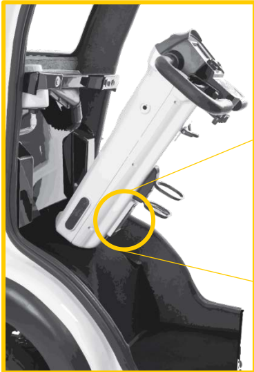
Figure 11 - Fuse box located on tiller
