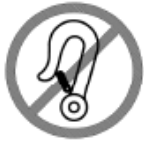
Figure 7 – Symbol for prohibition not intended to be used as a seat in a motor vehicle
