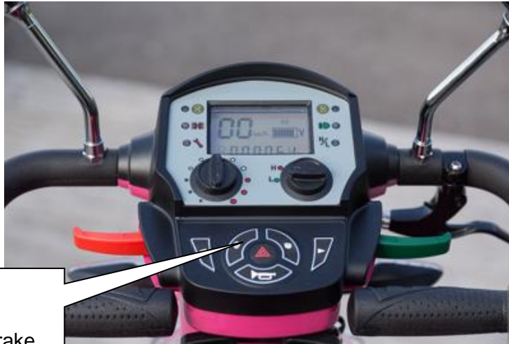
Figure 6: Electric button for Freewheel mode
