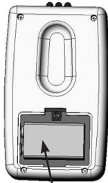
9V battery (access panel removed)
