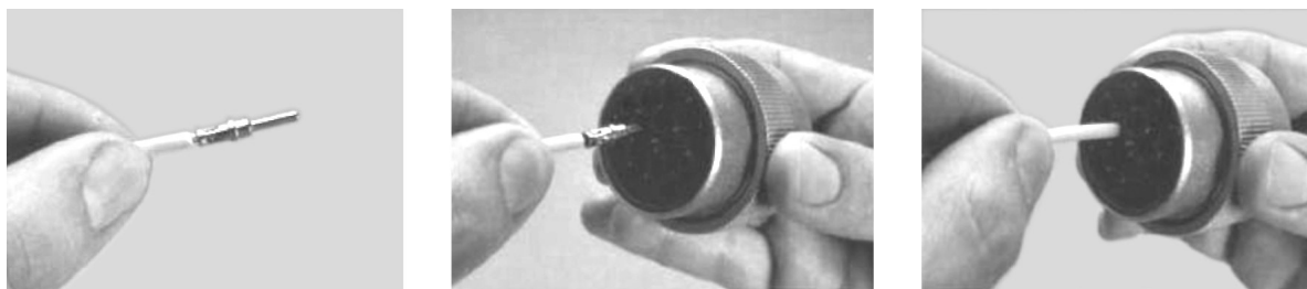
Figure 7-14. HD/HDP Contact Installation
