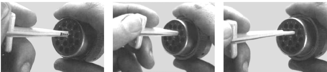
Figure 7-16. HD/HDP Contact Removal
