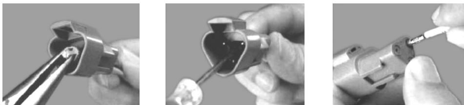
Figure 7-13. DT/DTP Contact Removal
