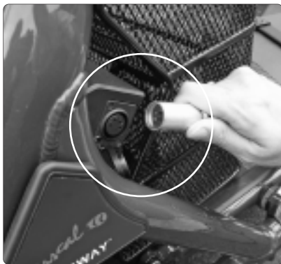
Charging Point (on rear chassis)
