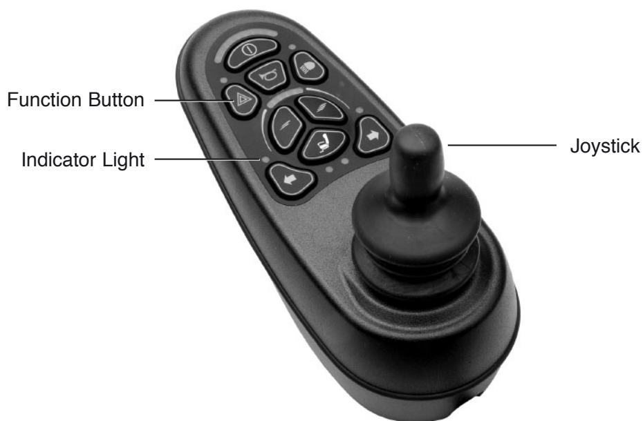
VR2 control panel overview
