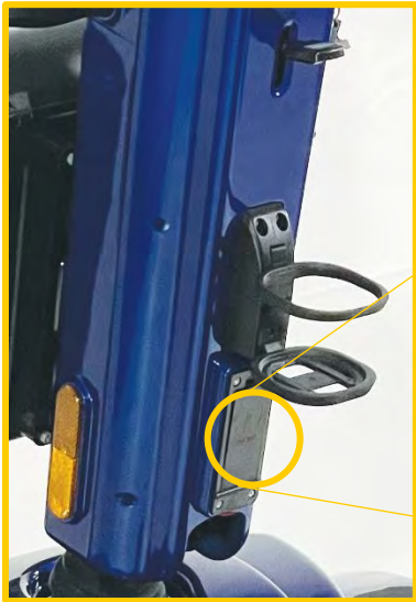
Figure 16 - Fuse box location
