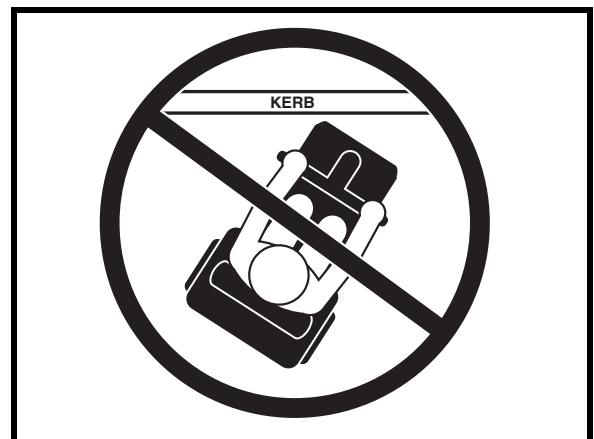
Figure 3A. Incorrect Kerb Approach
