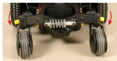
Position for disengagement - pushed down
