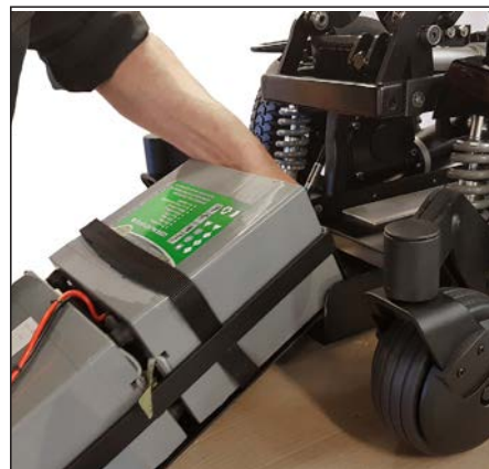
Make sure that the plug is nearest the entrance. Slide in the battery box.
