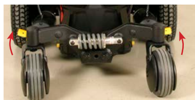
Normal position for driving - pushed up
