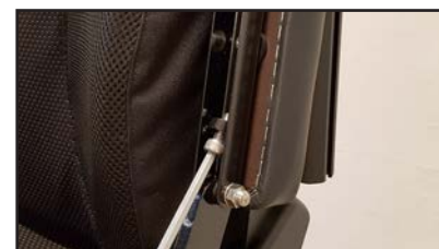
When the screw is screwed in, the armrest is angled downwards and screwed outwards, the armrest is angled upwards.
