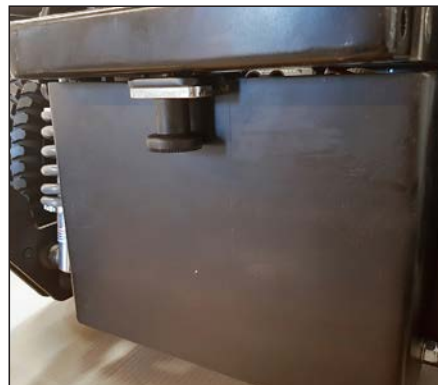
Pull the handle down and flip the cover out.
