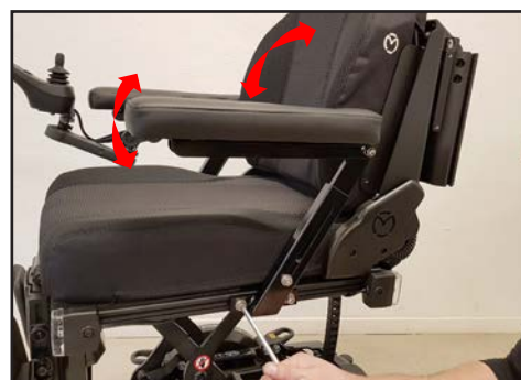
When the screw is screwed in, the armrest is angled downwards and screwed outwards, the armrest is angled upwards.
