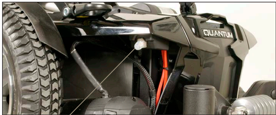
The automatic fuse is placed here.
