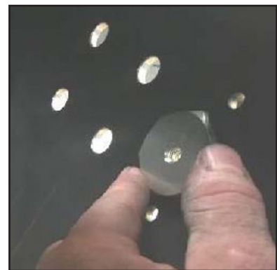
Place the nuts in the predrilled holes.
