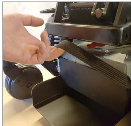
Pull the battery strap to slide out the battery box.
