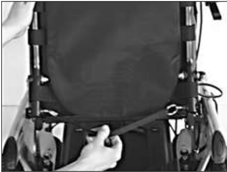
Fig. 46 Folding the backrest down
