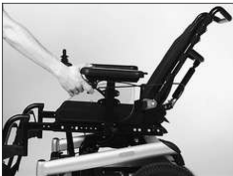
Fig. 26 Adjusting the back angle manually
