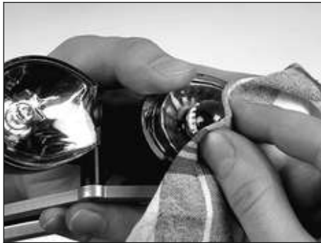
Fig. 53 Replacing the front direction indicator bulb
