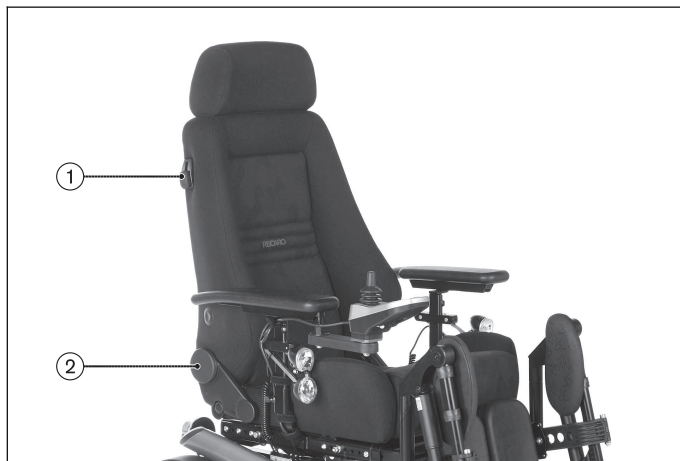
Fig. 4 Adjusting the Recaro® seat angle
