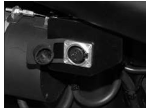
Fig. 19 Charging receptacle on power wheelchair
