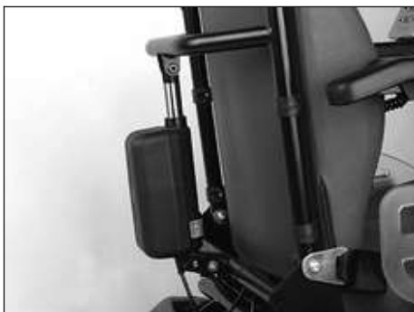
Fig. 22 Power back angle adjustment
