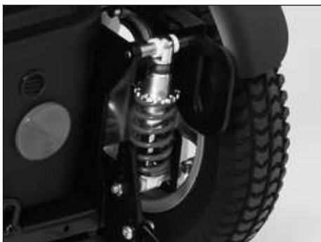
Fig. 42 Drive wheel suspension
