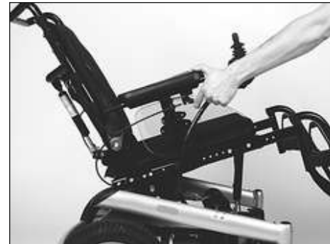
Fig. 25 Tilting the seat manually
