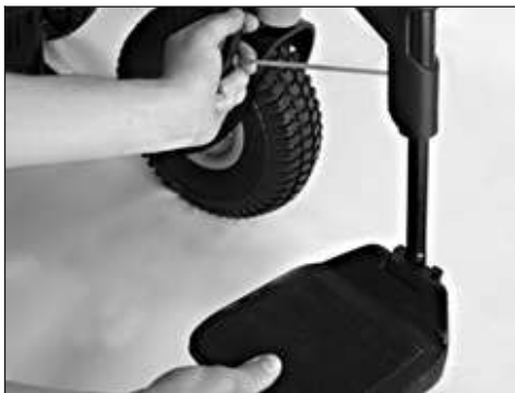
Fig. 7 Adjusting the lower leg length (standard footrest)
