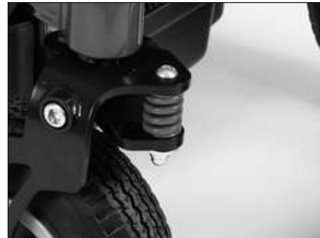
Fig. 41 Steering caster suspension
