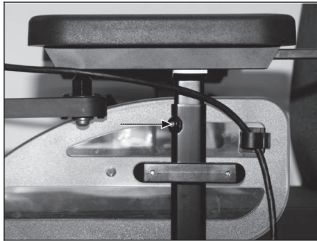
Fig. 5 Allen head screw for height adjustment
