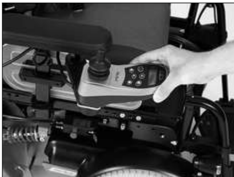
Fig. 36 Swing-away control panel holder with removable control panel
