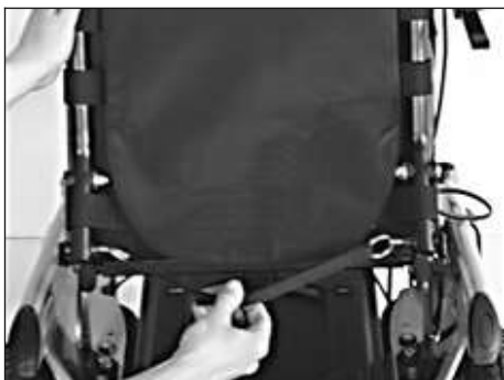
Fig. 3 Adjusting the back angle
