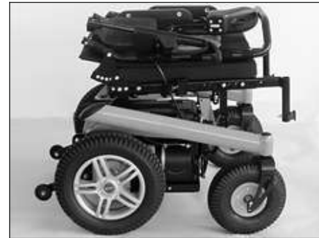
Fig. 45 Power wheelchair with reduced transportation size
