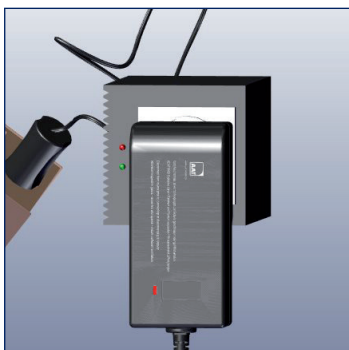
LED is red = batteries are charging.
