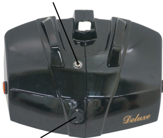
Battery Charging Socket
