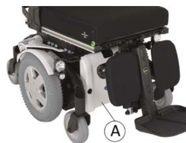
Batteries behind front shroud (A)
